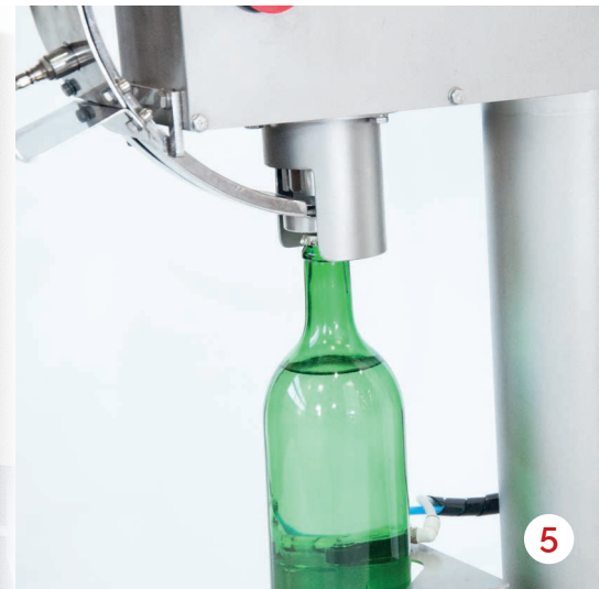
Caption: 1) Carbonator pump, 2) Pneumatically-actuated filling unit, 3) Run-dry protection, 4) Pressure regulation unit for CO 2 & connection for carbonated liquids, 5) Crown caps closing machine
