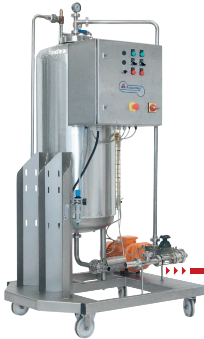
Caption: 1) Carbonator pump, 2) Pneumatically-actuated filling unit, 3) Run-dry protection, 4) Pressure regulation unit for CO 2 & connection for carbonated liquids, 5) Crown caps closing machine
